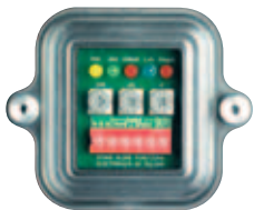
DIL switches to set Stand Alone functions and rotary DMX address switches
