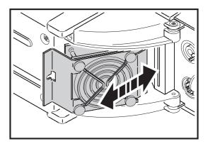
Figure 4: Cooling fan removal
