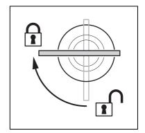
Figure 2: Locking a quarter-turn fastener
