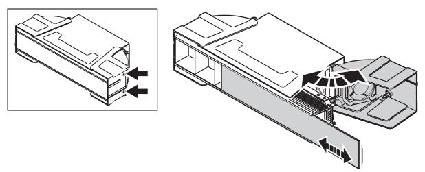
Figure 5: Installing and removing the diffuser front
