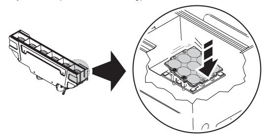
Figure 6: Lens removal
