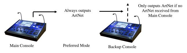
In "Equal mode" all consoles on the network are set to "Hot take-over". At any one time, one of the consoles will run as the master, with all universes enabled. If that console fails, one of the others will take over. It is recommended that you set the "Hot take-over detect time" to different values on each of the consoles to avoid conflict conditions.
