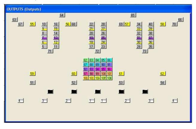
In the Outputs Window, select View Plan and View Hd Nos. Press Grid Size and enter a matrix size for your lighting rig - e.g. 30/20 gives a 30 by 20 grid.
