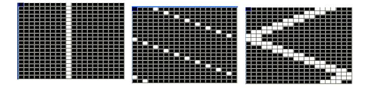
Vert random, Horiz random – enable random movement of elements across the grid. Modify the mode to change thickness of the elements and offset to change the frequency. With this FX it is possible to generate snow and rain type FX.
